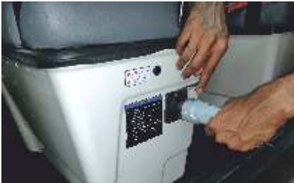
Figure 24: Correct way to insert and remove the connector
