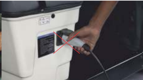
Figure 25: Wrong way to remove the connector
