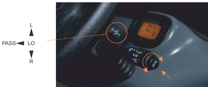
Figure 15: Lights and horn switches
